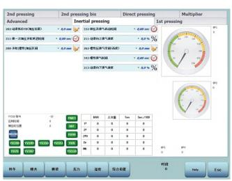
The new generation of advanced PC-PLC control system makes the operations faster, simpler and clearer. The cycle of the press is controlled with a special CPU which connects the system to each control unit box via cables.
